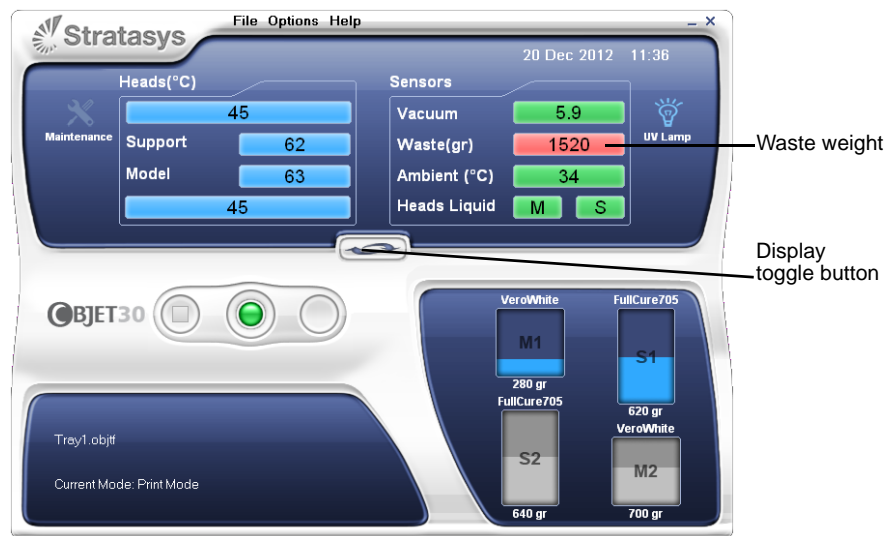
Figure 6-108: Printer interface, showing waste weight (red background indicates operator alert)
