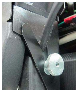
Figure 6-49: UV-lamp cable in place after securing the assembly
