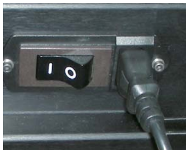
Figure 6-2: Main power switch and cable
