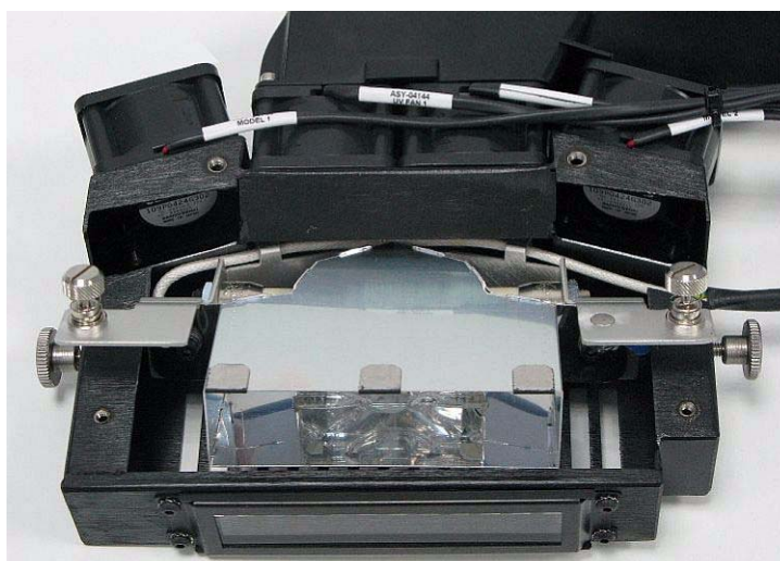
Figure 6-100: Removing the UV reflector from the UV assembly
