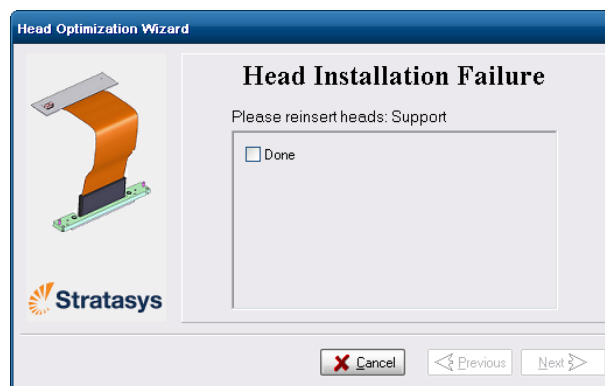
Figure 6-80: Incorrect-installation screen, showing which head(s) to re-insert
