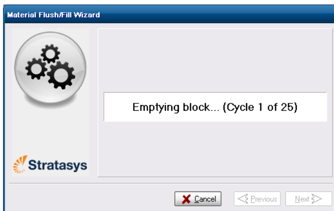
Figure 6-29: Flushing cycles in progress
