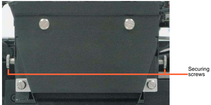
Figure 6-44: UV-lamp-assembly securing screws
