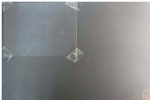
Figure 6-51: Positioning the transparency on the build tray
