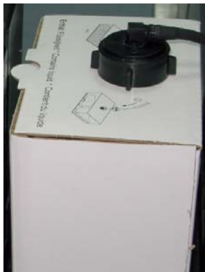
Figure 6-110: Waste container with drain tube attached
