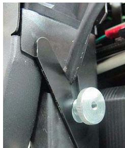
Figure 6-102: UV-lamp cable after replacing the assembly
