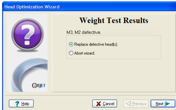
Figure 6-56: Defective print heads found
