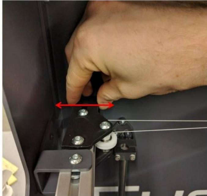
**If One Cable is Loose, or You are Adjusting the X Axis Square:**
