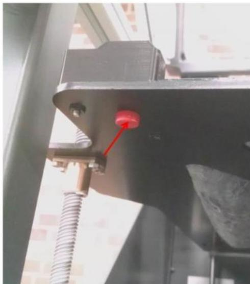
Turning it **counter-clockwise** will **lower** the bed corner. And turning it **clockwise** will **raise** the bed corner.
