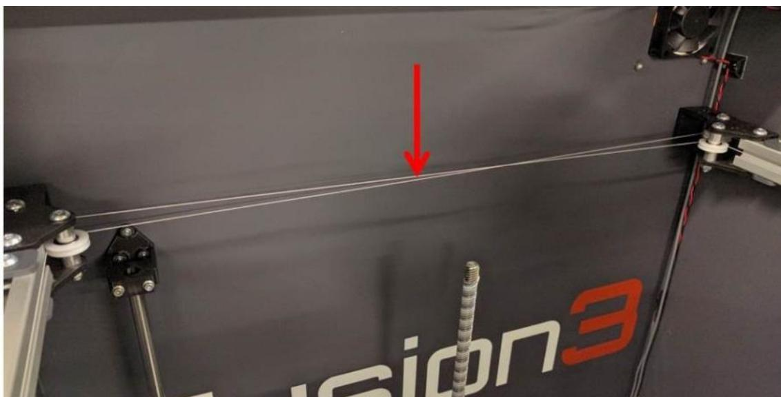
Use a light finger touch on the cables to ensure they are not slack. A wide range of tension is acceptable; as long as the cables are not actually loose they are fine.
