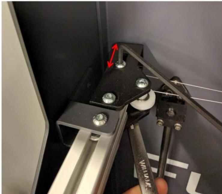
Once you adjust the pulley, tighten the screw and re-check the square.
