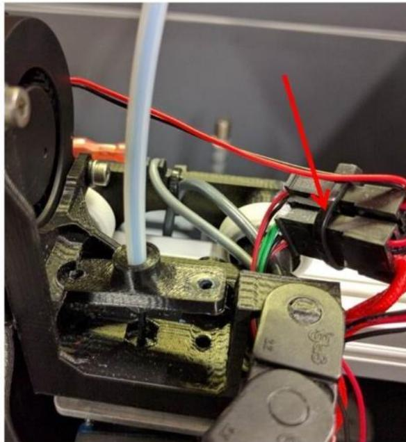
Clip the zip tie holding the print head wires to the print head assembly.
