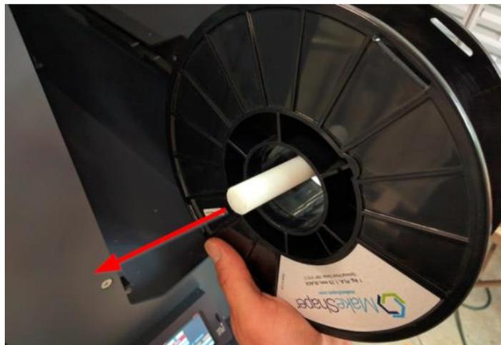
Orient the spool so the filament pays off the front side (or underneath) of the spool.
