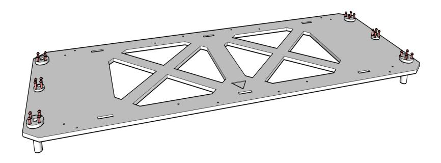
Mount the (4) LM8FLUUs through the corners of BFP-10. Mount the T8 nuts through the middle holes. Make sure the arrow is facing you and on top.
