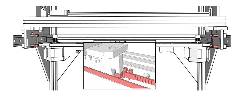
Mount the part we assembled in the last step to the blocks on the linear rails using the M3 hardware. **Make sure BFP-19 is on the front end.**
