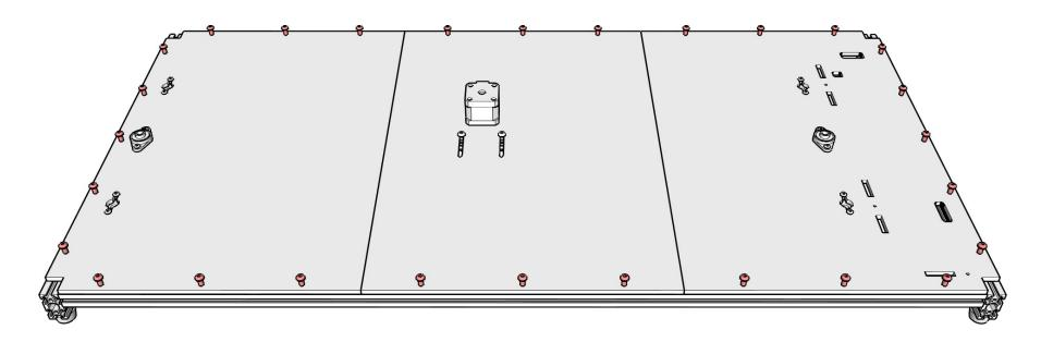
Mount the (3) lower panels using the M5 hardware. Make sure the orientation is correct.
