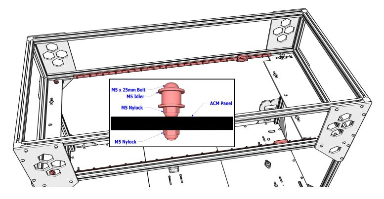
Mount the (2) idlers using the M5 hardware. Make sure the idlers spin free. Mount the (2) 800mm linear rails between the upper plates using the M3 hardware in every other hole.
