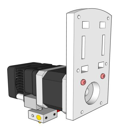
Remove the top 2 bolts on the back of the stepper. Mount the stepper to BFP-SD02.
