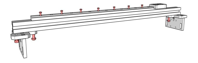
Mount the assemblies from the last step to the ends of the 500mm 2020 using the M5 hardware. Make sure the hex head bolts are on the ends. Mount the 400mm linear rail 50mm from either end of the 2020 using the M3 hardware in every other hole.
