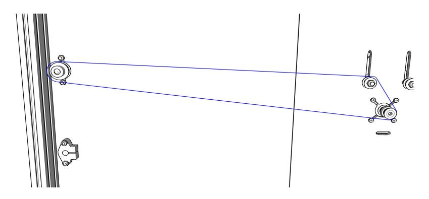
Route a belt loop as shown. Tighten by moving the idler. Repeat for other side. Adjust pulleys as needed.
