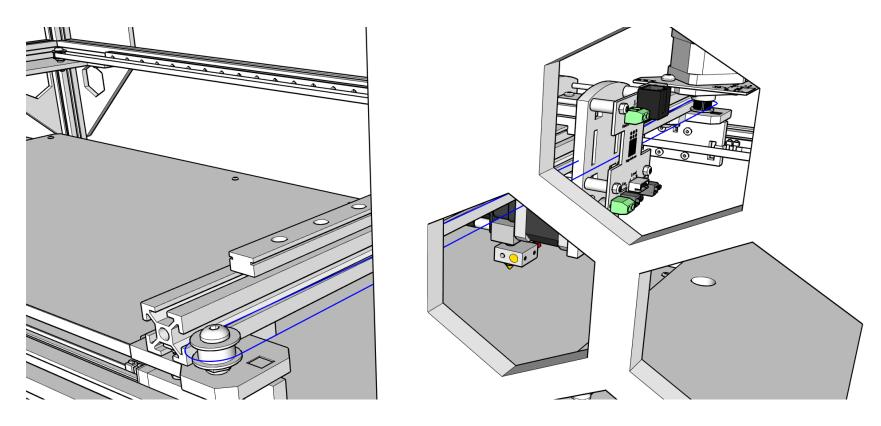
*Tightly* install the Y belt as we did earlier with the X belts. Attach the left side of the loop to the carriage with the right side of the loop behind the PCB. Adjust tension by moving the Y stepper assembly.
