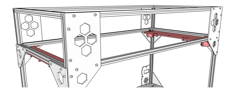
Mount the assembled BFP-08 and BFP-09 to the underside of the middle 2020 using the M5 hardware.
