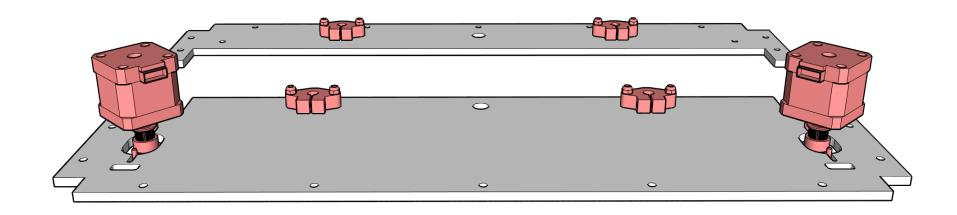
Mount the (4) KFL8s to BFP-08 and BFP-09 using the M4 hardware. Mount a pulley upside-down to each stepper, flush with the end. Mount the steppers using the M3 hardware. All of the bolts go on the bottom. Make sure you face the stepper plugs the correct direction.
