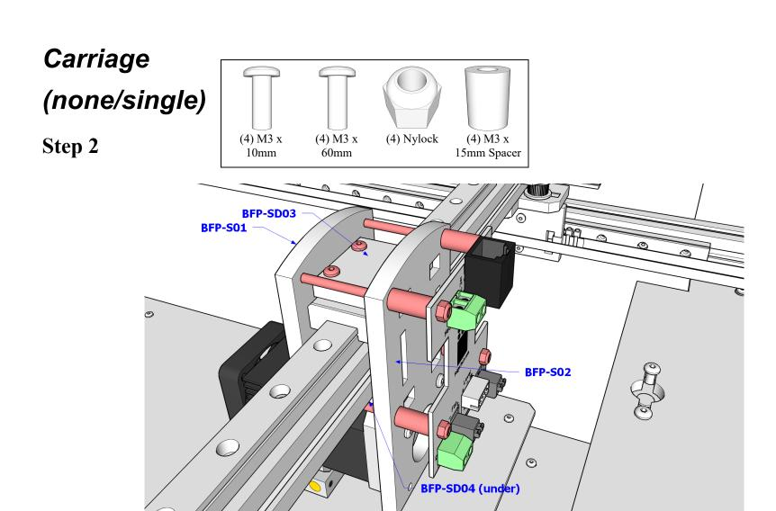
Mount BFP-SD03 to the linear block. Assemble BFP-S01, BFP-S02, BFP-SD04, and the carriage PCB using M3 hardware and spacers. The PCB is on the right hand side of the gantry.
