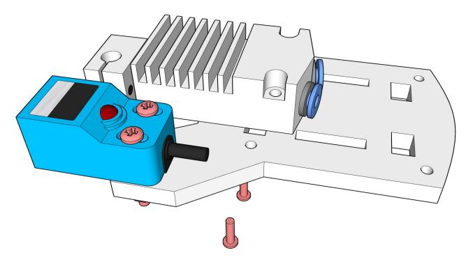
Mount the sensor in the center of the slots using the supplied hardware. Mount the dual hotend using the top set of holes that don't go through.
