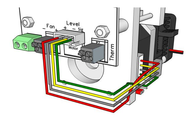
Using a short stepper cable, plug the extruder stepper into the carriage PCB.
