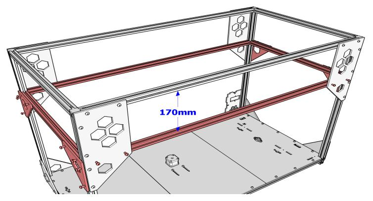
Mount (2) 1000mm 2020 and (2) 500mm 2020 using BFP-02s and M5 hardware. Verify the top 2020 to middle 2020 spacing is 170mm all the way around.
