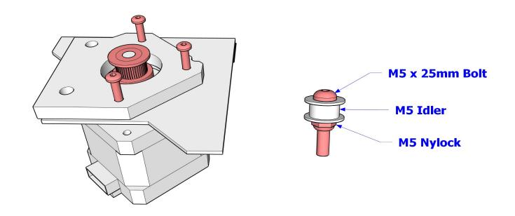
Mount the pulley to the stepper flush with the end. Stack BFP-20 on top of the gantry board and mount to the stepper using the M3 hardware. Assemble the Y idler using the M5 hardware.
