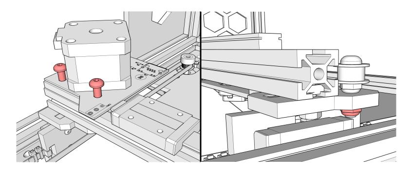
Mount the Y stepper assembly to the rear end of the gantry using M5 hardware. Mount the Y idler to the hole in BFP-19 using the M5 nylock.
