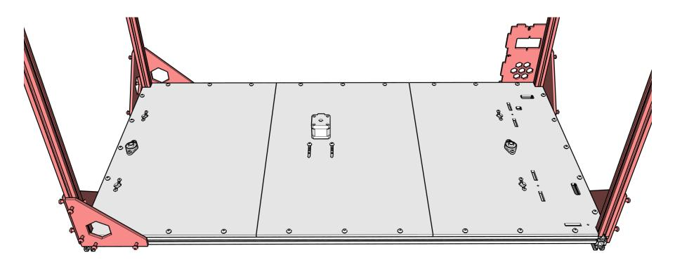
Mount (2) 700mm 2020s on the left with BFP-01s. Mount (2) 700mm 2020s on the right with BFP-03, BFP-04, and BFP-12. Make sure the joins are square and flush against the lower frame.
