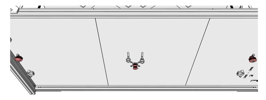
Flip the printer onto it's back or prop it up and mount the pulleys as shown. Make sure the left one is upside-down. You may need to adjust the T8 lead screws.
