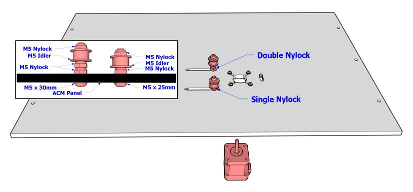
Mount the stepper to BFP-06 using the M3 hardware. Assemble and mount the (2) idlers as shown using the M5 hardware. Make sure the idlers spin free.
