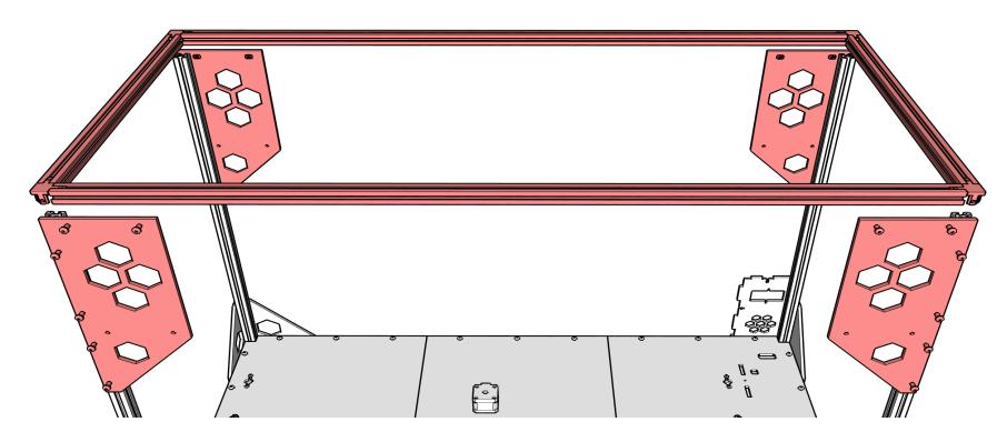
Assemble the top frame with (2) 1000mm 2020 and (2) 500mm 2020 using (4) 3-way corners. Mount the top frame to the uprights using BFP-02s and M5 hardware. **Make sure the joins are square and flush.**
