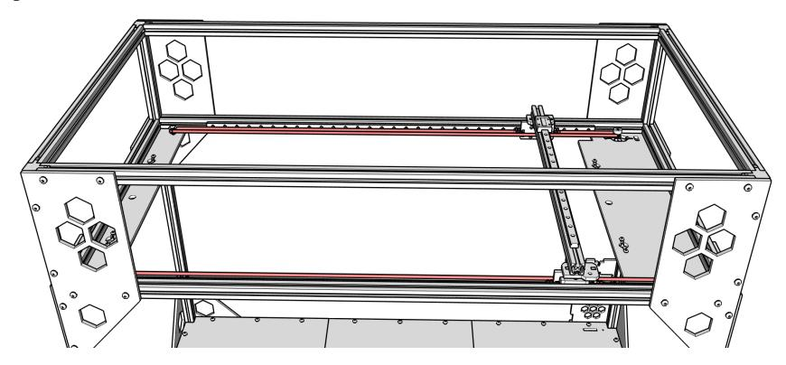
Install the X belts with the teeth against the pulleys. Trim and secure to the tabs with cable ties as shown. Tighten them by adjusting the steppers.
