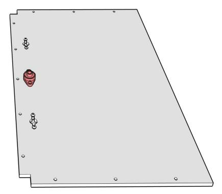
Flip the panels over and mount the (2) KFL8s. The bolts go on the top. Make sure the center of the KFL8s swivel in the socket. You may need to add some oil and work them a bit.
