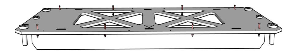
Mount the BFP-11s to BFP-10 using M3 hardware.
