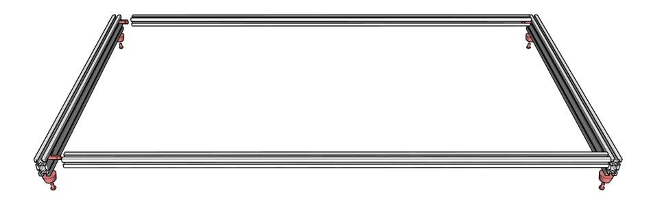
Assemble the lower frame with (2) 1000mm 2020 and (2) 540mm 2040 using the internal L brackets and grub screws. Mount (4) rubber feet using the M5 hardware. Make sure the joins are square and flush.
