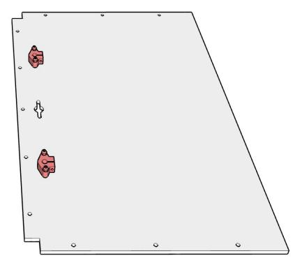
Mount the (4) SHF8s to BFP-05 and BFP-07. The bolts go on the bottom with the nut on top.
