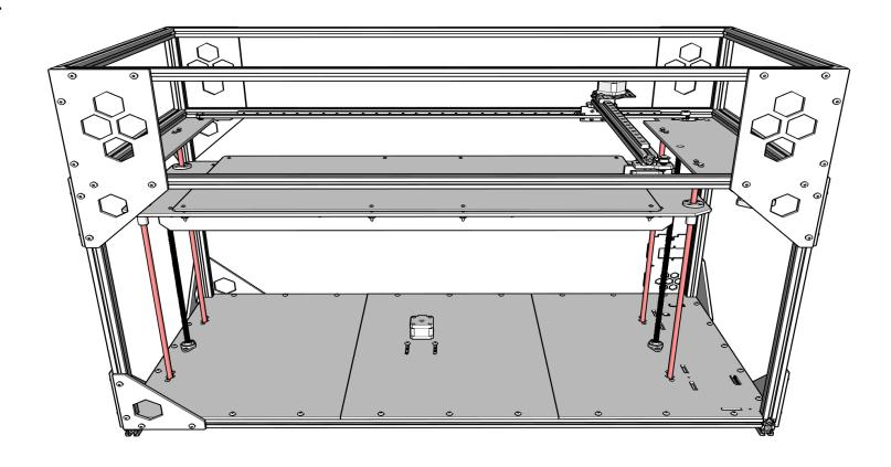
Mount the bed assembly to the printer by sliding (4) 500mm PCRs into the corners and thread (2) M8 lead screws into the middle. Tighten the SHF8s to hold the PCRs in place. Tighten the set screws on the KFL8s to hold the lead screws in place.
