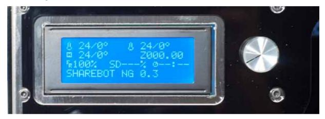
The first line contains the actual extruder temperature followed by one set; If the extruders are two, the first is on the left while the latter is right. What is used as the primary extruder is the one on the right. The temperature is in degrees Celsius.
