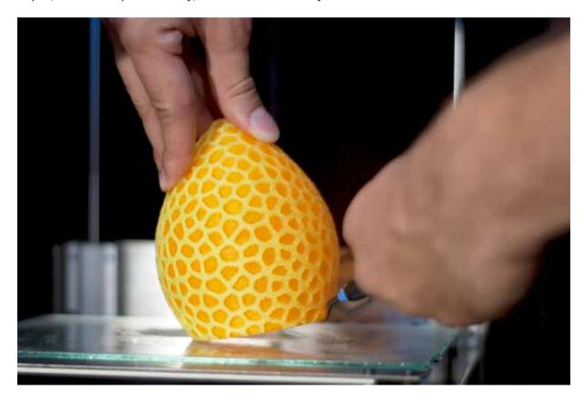
As advice, avoid using the same piece as an element to force (pulling) or lever (it) because it could break. If the printed object has a high surface you can remove the Print plate and place it under warm water, allowing the dissolution of Hairspray and a detachment of the piece easier.
