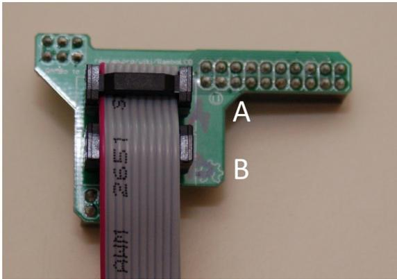
Fig. 17.10-3B: Red or Blue Display PCB cabling.
