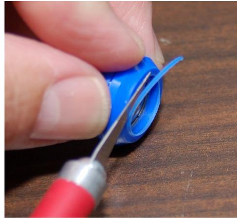
*Fig. 9.1-5 Removing the edge.*
