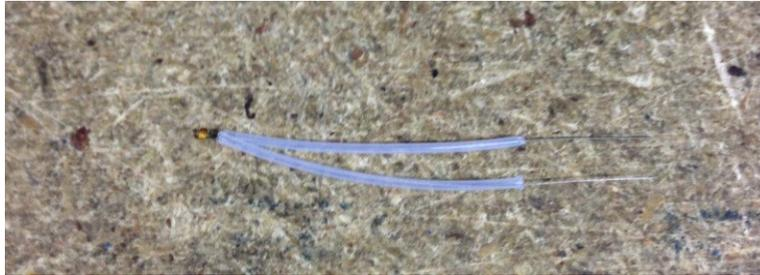
*Fig. 3.1-6: Thermistor with PTFE sleeves installed.*
