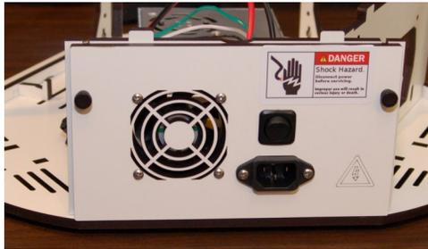
*Fig. 6.6-8: Power supply install complete.*
