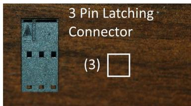
The 3 pin latching connectors can be found inside the RAMBo parts baggie (marked “RAMBo v1.3 Kit” or similar).
