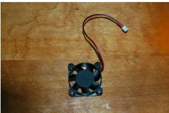
[ ] (1) 40x40x10mm 12VDC fan. RAMBo cooling fan. [26177]
