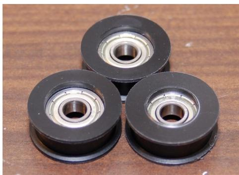
*Fig. 8.5-1: Assembled bearing sleeves.*
