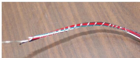
Fig. 7.1-3: Correct fish-wire wrapping.
