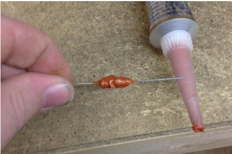
*Fig. 3.1-3: Coating the heating resistor with RTV.*
