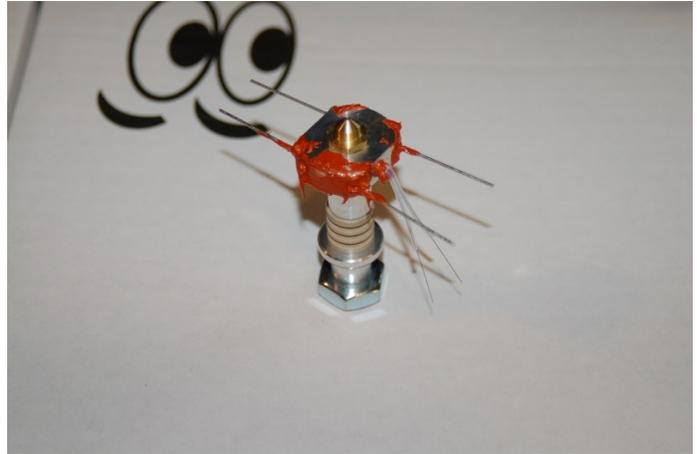
*Fig. 3.1-10: Hot end plugged into the cardboard box for curing.*
