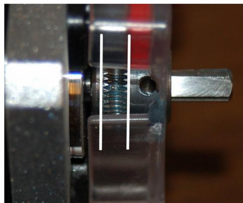
Fig. 10-5: Hobbed gear alignment.
