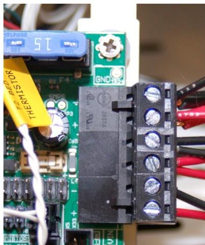
Fig. 17.8-8: Power connector attached.
