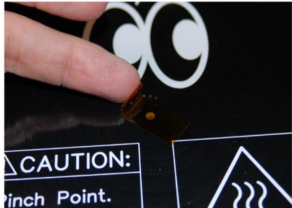
Fig. 4.1-1: Covering the thermistor hole.
