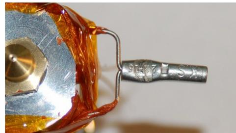
Fig. 11.3-7: Crimp installed.
