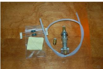
[ ] (1) Hot End Kit. Includes hot end, heating resistors, thermistor, PTFE sleeve for thermistor, PTC fittings and PTFE bowden tube. [68394]
