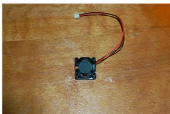
[ ] (1) 25x25x10mm 12VDC fan. Used to cool the PEEK section on the hot end. [26309]
