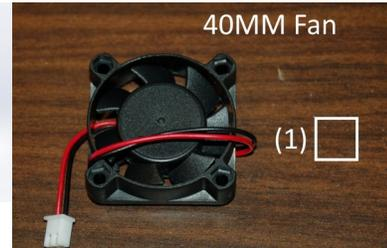
You'll also need two short wire ties in order to attach the fan to the back of the RAMBo mounting plate.
