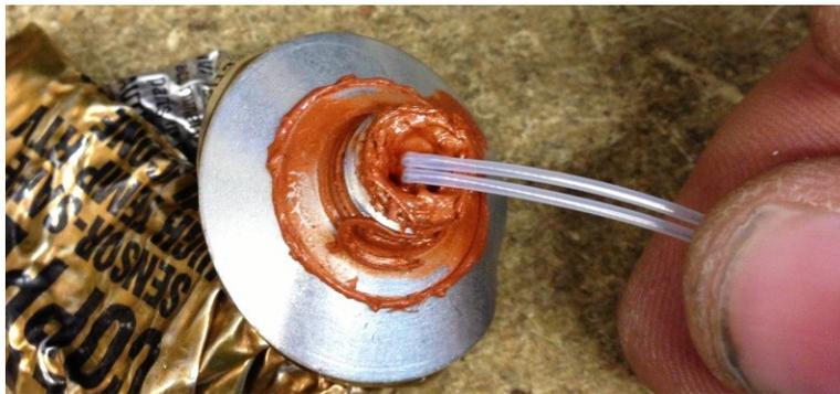
*Fig. 3.1-8: Coating the thermistor with RTV.*
