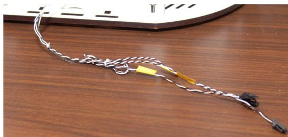
Fig. 17.3-4: Finished end-stop wiring.
