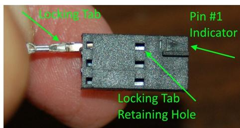
Fig. 17.3-2: Setting the first connection.
