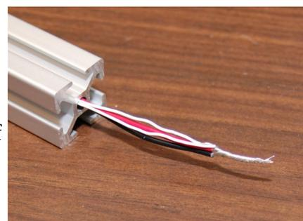
Fig. 7.1-5A: 18/26ga wire routing.
