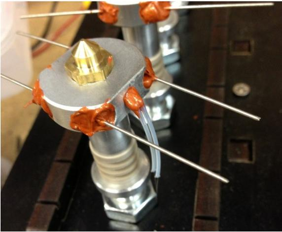
*Fig. 3.1-9: Thermistor installed.*
