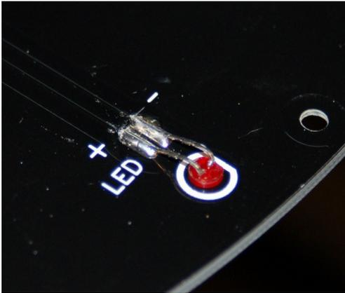
Fig. 4.2-5: Soldered and trimmed!
