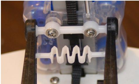
*Fig. 12.2-4: Carriage end spring.*
