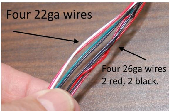
Fig. 7.1-2: Z Axis wires.
