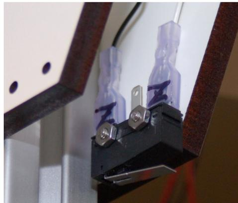
Fig. 8.7-3: Z axis end stop switch wired.
