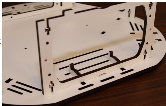
*Fig. 6.4-4: Front vertical support installed.*
