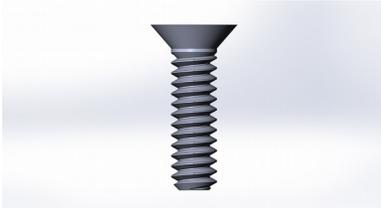
[ ] (12) #6-32, 1/2” 18-8 Stainless Steel Flathead screw. Used inside of base and top side plates, to retain acrylic panels and the three end-stop triggering screws installed in the Cheapskate U-Joint mounts. [30135]
