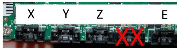
Fig. 17.8-5: Stepper motor connectors.
