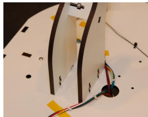
*Fig. 14.1-6: Spool holder support mounted.*
