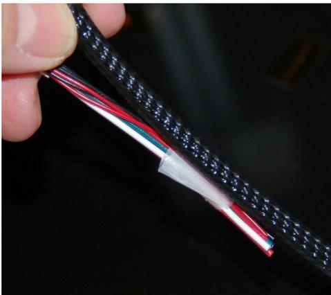
*Fig. 11.1-1: Wires and mesh loom.
