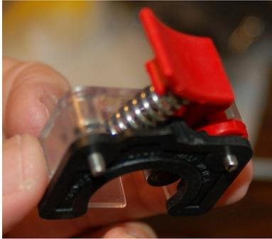
Fig. 10.1-2: Filament tensioner.
