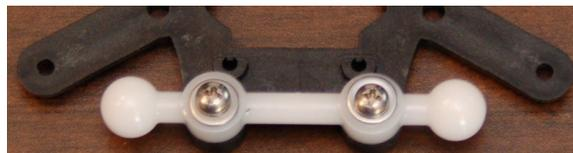
Fig. 12.1-2: Ball Joint Arm fixed in place.
