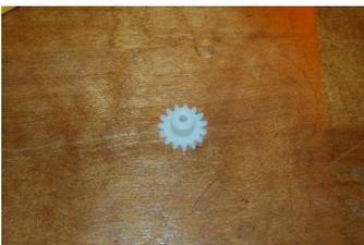
[ ] (1) 15 Tooth Gear. Used for manually operating extruder motor.
