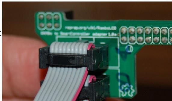
Fig. 17.10-3A: “A” & “B” cables installed (White PCB only!).
