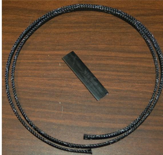
*Mesh wiring loom and heat shrink tubing.*
