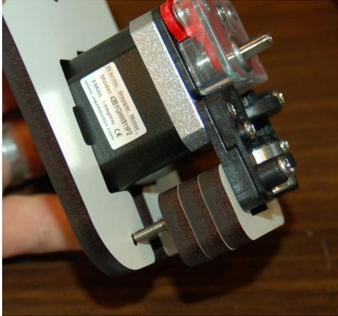
*Fig. 10.2-5: Fitting the EZStruder to the bracket.*
