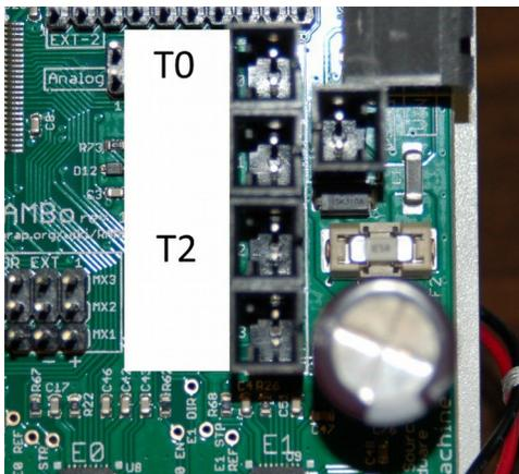
Fig. 17.8-3: Thermistor connectors.
