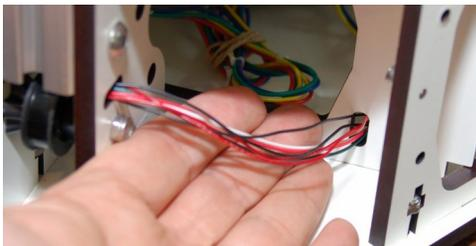
Fig. 7.2-5: Z Axis wiring routed forward.
