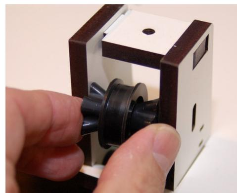
*Fig. 8.5-2: Positioning the idler assembly.*
