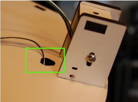
Fig. 8.7-1: Z axis end stop wire hole.
