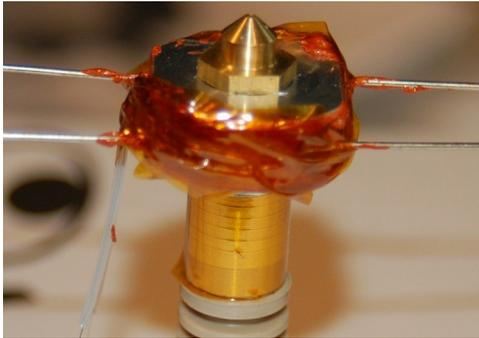
Fig. 11.2-2: Heater block and hot section wrap.
