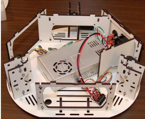
*Fig. 6.8-1: X & Y Tower supports installed.*
