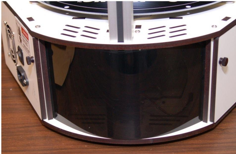
*Fig. 18.3-3: Z Axis cover installed.*
