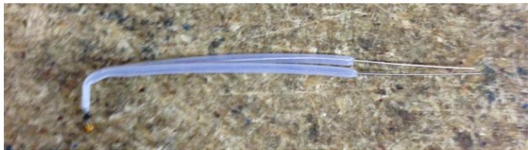
*Fig. 3.1-7: Bending the thermistor.*
