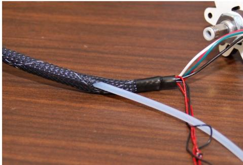
Fig. 11.5-1: Bowden insertion point.
