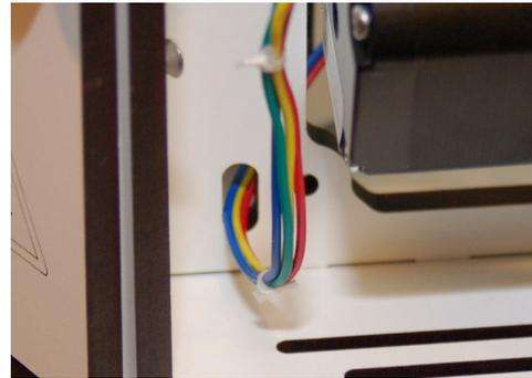
*Fig. 6.8-2: Z Axis motor wire route.*
