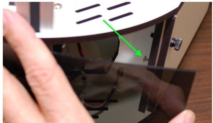
*Fig. 18.3-2: Setting the Z axis cover into place.*
