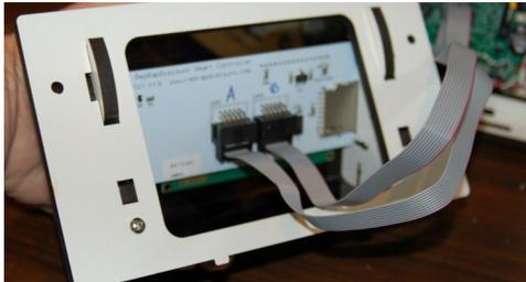
*Fig. 18.1-2: LCD controller cables installed.*
