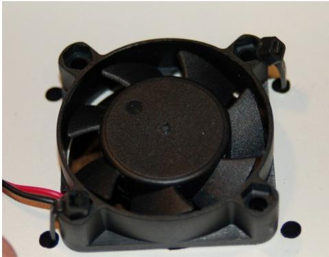
Fig. 17.1-3: Fan installed.
