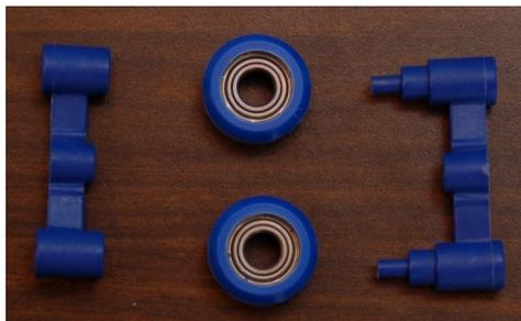
*Fig. 9.4-1: Spring arm components.*
