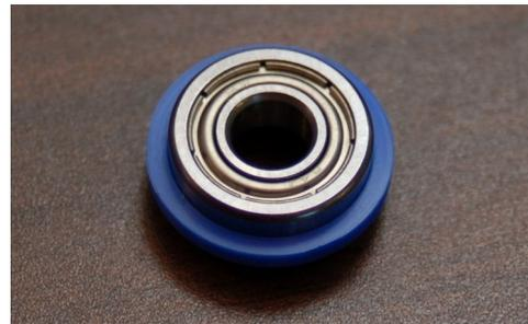
*Fig. 9.1-2: Pressed into the sleeve.*
