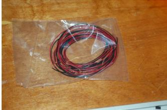
[ ] 15 feet, 26ga, Black & Red wire. Used for hot end PEEK and part fans. [26728, 26726] (Supplied as 30ft)
