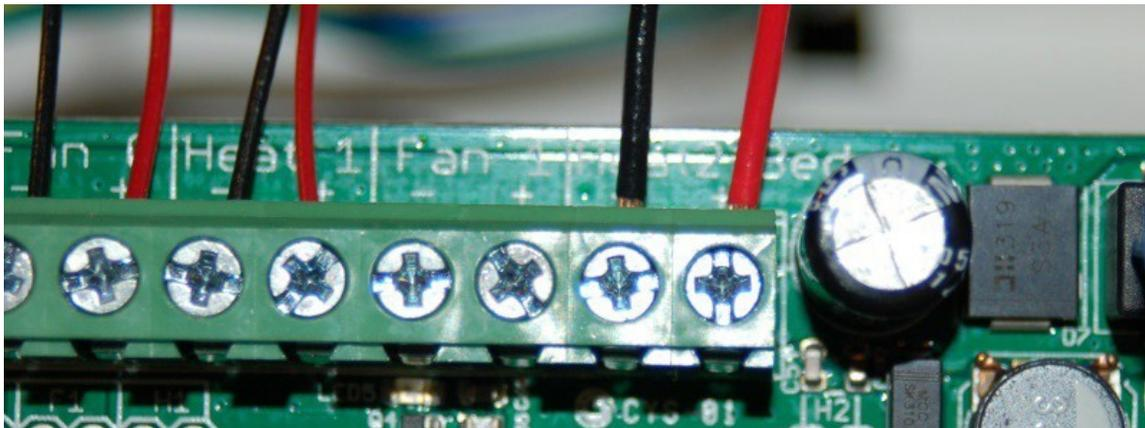
Fig. 17.7-4: Heated bed wires installed.
