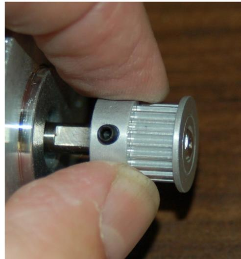
*Fig. 5.1-2: Gear and grub screw aligned.*
