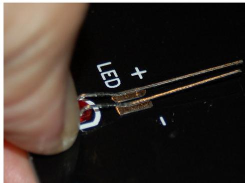
Fig. 4.2-4: LED ready to solder into place.
