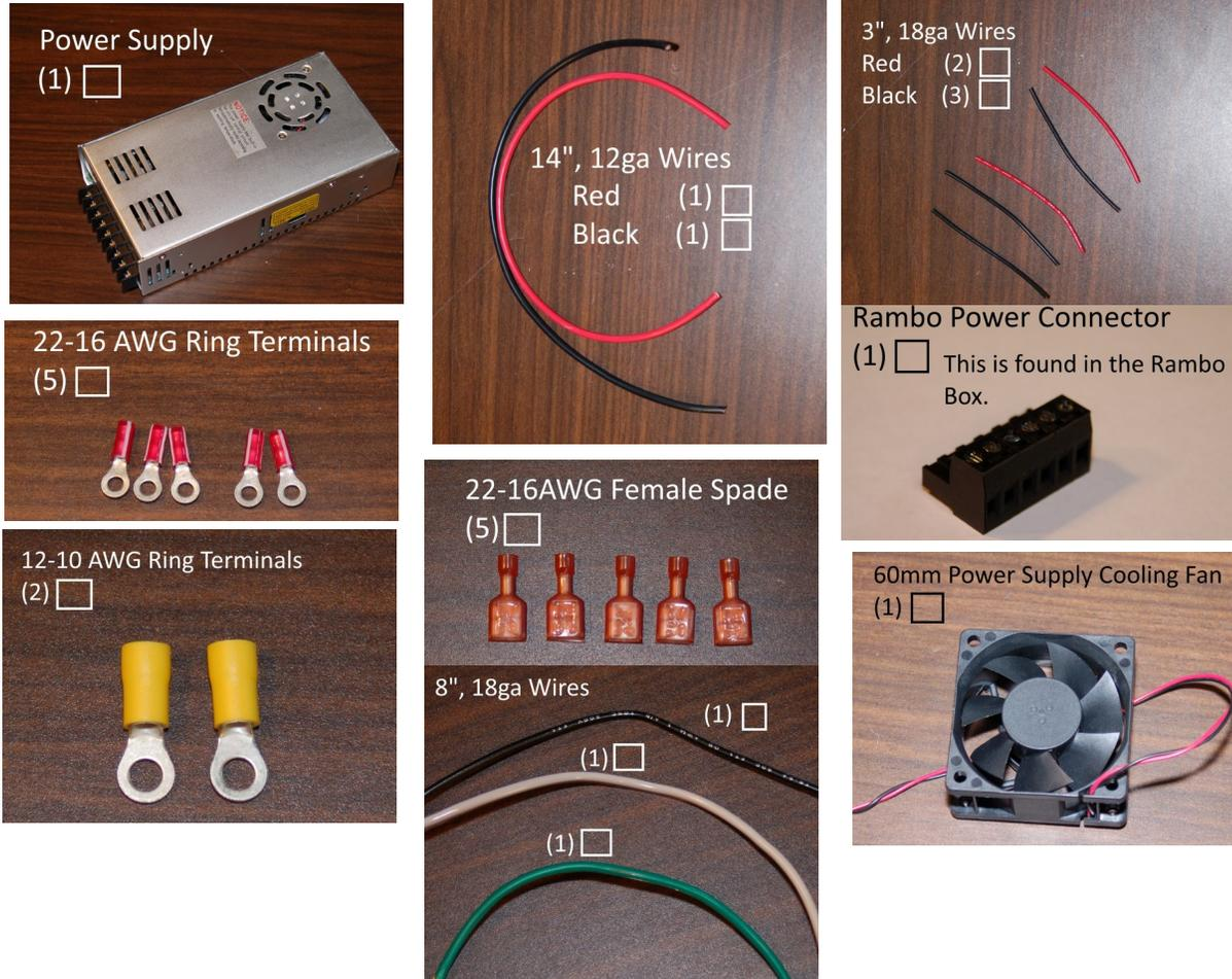
Your Rostock MAX v2 uses a 12 volt, 29 amp industrial power supply to provide power to the RAMBo controller, the Onyx heated bed and the hot-end. The power supply won't be installed until a later step, but there's some prep work that you can do now.
