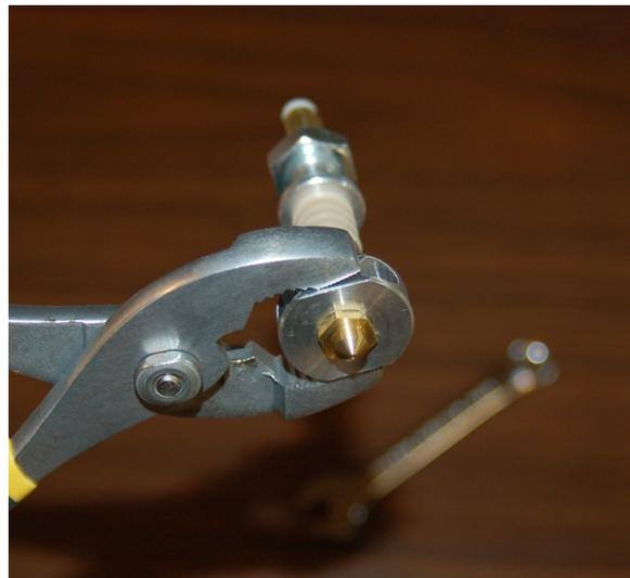
*Fig. 3.1-1: Tightening the nozzle.*
