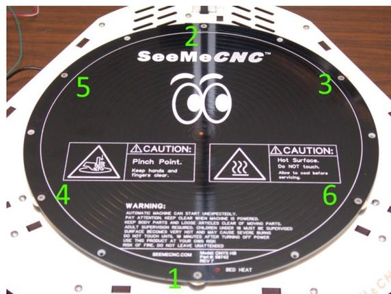
Fig 15.1-5: Screw tightening pattern.
