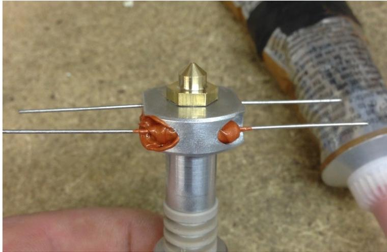
*Fig. 3.1-4: Resistors installed in the hot end.*
