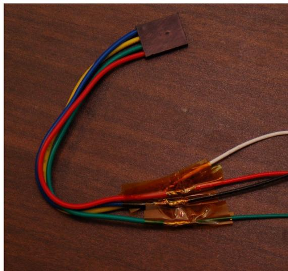
*Fig. 17.6-1: Extruder stepper connector soldered on.*
