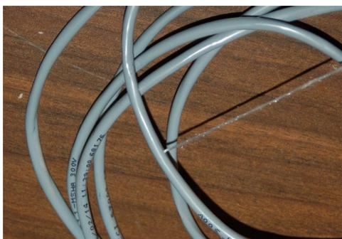
Fig. 7.1-1: Splitting the outer jacket.
