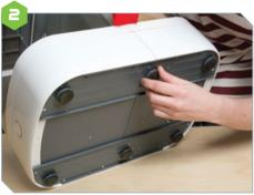
It is preferable, though not essential, for the printer to be level during operation. Check by placing a spirit level on the base platform, and then adjust the feet as necessary: turn clockwise to raise them, anticlockwise to lower them.
