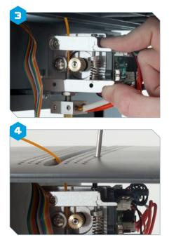
whether the filament is being held too tight or too loose. (This is a good time to familiarise yourself with the drive gear quick-release mechanism: squeezing the sprung tabs releases
