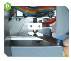
LEFT: Once you have reduced the gap between build plate and nozzle to a millimetre or less, use the calibration gauge to measure it. The gauge should just slide into the gap at all five points shown in the Calibration Setup window (image A).
