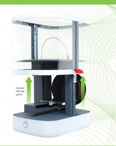
To raise the hood, grip both cloth tabs and lift. Lift the hood fully until you hear the click as it stops at the upper catches. You can now release the cloth tabs. To lower the hood, slide the upper catches towards you. Lower the hood fully until its lower frame rests squarely on the base plate.
