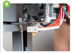
Offer the print head up to the attachment plate on the printer (above), making sure the lug on the print head (below) fits the hole in the plate. Affix the head using the two 18mm Allen bolts, taking care not to overtighten them.
