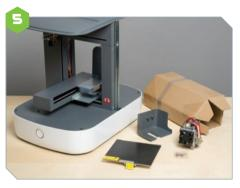
Carefully remove the cardboard accessories box from the gantry and check that it contains the following: print head (plus two Allen bolts), print head guard (plus one screw), build plate base (plus four countersunk bolts), and build plate.
