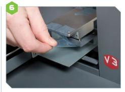
For added protection from damage during transit, the X- and Y-axis movement has been immobilised with a shipping bracket, which must be removed before operation. First, peel the adhesive tape off the base mounting block.
