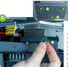
**LEFT:** Carefully turn the adjustment bolts to level the plate. For instance, to lower the right-hand side, tighten the right-hand bolt (marked R above). To raise it, loosen bolt R. To raise the back of the plate, loosen the centre bolt C; and so on.
