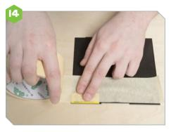
If you choose to tape the plate, we recommend 48mm-wide tape, rather than 24mm, to minimise the number of joins. Run lengths of tape over the plate, leaving enough to fold a little underneath at the ends. Don't overlap them. Instead, simply butt-join them, or leave a small (1–2mm) gap.
