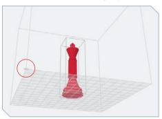
The lower front corner of the field has a small pad (circled, above); to reset the view, drag this pad back to its original location. Or click Reset to bring it back.
