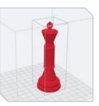
This dragging method only gives an approximate scale value. To scale more precisely, double-click on Scale to bring up a measurement panel, and then type in a scale factor. (This method is useful for scaling multiple identical prints.)
