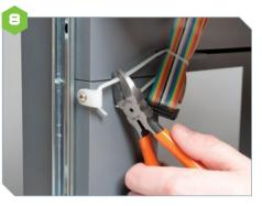
Cut cable ties from around the multi-coloured print head cable (above). You can remove the tie-retaining lug from the self-tapping screw on the gantry (below), but be sure to replace the screw securely afterwards.
