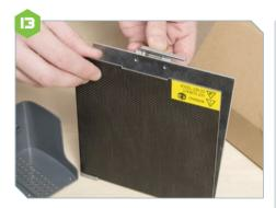
The build plate is attached to the build plate base for shipping. You'll need to unclip it in order to attach the base to the printer.
