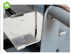
Using a Philips screwdriver and the four countersunk bolts, attach the build plate base to the printer, with the sprung clip at the front and the two catches at the back, as shown. Ensure the bolts are driven fully home so that the heads are not proud of the plate surface.
