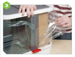
Peel the protective film from the hood frame window.
