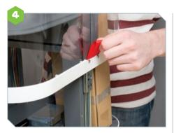
Gently raise the hood until it stops (above). Then, while sliding the retaining catches (see below), remove the hood fully from the gantry.
