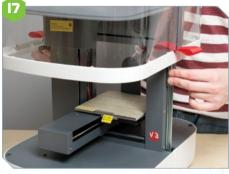
Reattach the hood. Guide the sides carefully into place so that they engage smoothly with the rails. Note also that the hood goes on only one way round, with the side-rails closer to the back of the printer than to the front.
