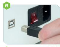
Plug the power adapter into the back of the printer, and the other end into a power socket.
