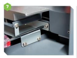
Next, remove the five screws – four at the back (see above), one at the front (below) – and take off the shipping bracket. You may want to keep the bracket somewhere handy in case you need to transport the printer, i.e. if moving house.
