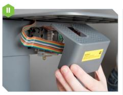
Offer the print head guard up to the print head, ensuring the tubular sockets on its inner face (below) engage with the two posts projecting from the print head. As you do this, make sure the multi-coloured cable wraps around to the left and is kept above the two posts.
