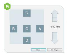
LEFT: In the Calibration Setup window, use the up/ down arrows to raise or lower the build plate. In the Windows version shown here, each three-part arrow enables you to adjust the plate height in graded increments (10mm, 1mm, or 0.1mm). The total travel height is displayed between the arrows.
