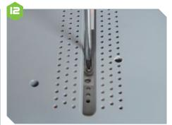
The print head guard is secured with a single Phillips screw. Access is via the slot in the printer top. Take care not to overtighten it.
