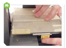
Affix the build plate to the plate base, first engaging the two rear recesses into their holders and then slotting the front recess into the spring-loaded clip. The design allows the plate to detach without damage in the unlikely event that the plate is driven up into the nozzle.
