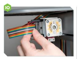
Insert the multi-coloured print head cable into the socket on the print head. It can be inserted only one way round. Ensure the plug is fully seated in its socket.
