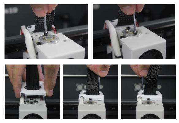
**13.** Insert the teflon tube until it stops, making sure it is well placed. Put back the black clip and the black piece.
