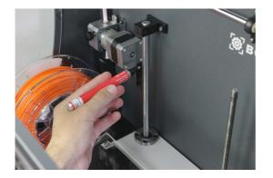
**4.** Clean grease and dust from the Z-axis motor spindle with paper or a cloth. Turn the spindle manually to access its rear.
