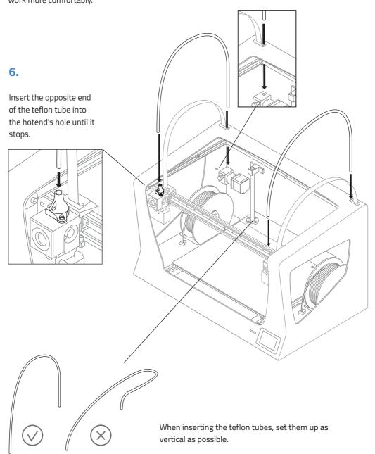
Attach the teflon tubes with the clips.
