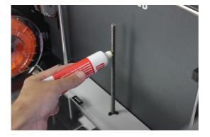
**6.** Turn on the Sigmax and from the LCD screen, go to *Utilities --> Maintenance --> Move printing surface.* Raise and lower the platform twice to evenly distribute the oil and grease. Finally, remove the remnant grease.
