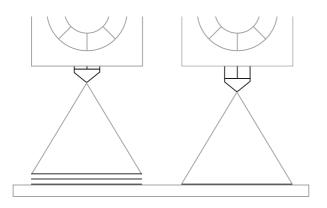
The Sigmax automatically corrects the offsets when printing in Duplication/Mirror modes. However, this correction distorts the first layer of the model by repeating it as many times as needed. To avoid such distortion there are different options:
