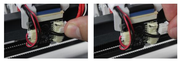
**10.** Remove the old hotend and place the new one, connecting it at the back of the toolhead carriage.
