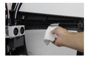
**9.** Clean the guides with the solvent pencil, making sure that it does not drip with special emphasis on the superior and inferior faces.
