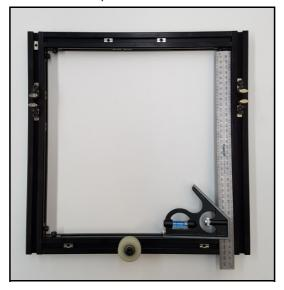
All corner joints must be at 90 degrees (perpendicular). Left and Right rails must be parallel as must the front and rear rails. Use a measuring tape or ruler to make sure that the distance between each set of rails remains constant from end to end – even if this results in a slight gap at one end where extrusion pieces meet.
