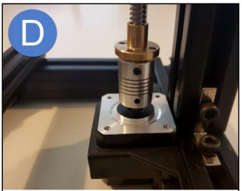
Note the gaps between the rings of the coupler. This is how it looks when grub screw is loose.
