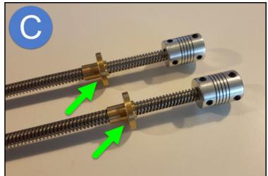
Place the Couplers (with Lead Screws Fitted) onto the Z Motor Shafts making sure that one of the grub screws is aligned with the flat on the shaft of the Motor.
