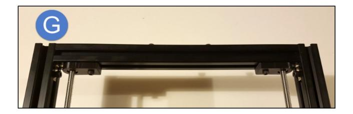
Take the remaining two M6 x 10mm Bolts and secure them in the two Sliding Nuts on the top of the Gantry. These will be utilised later for the Spool Holder Brackets.
