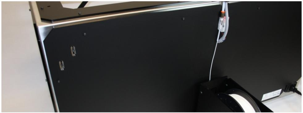
Now that the filament is inserted, dock again the teflon guide.
