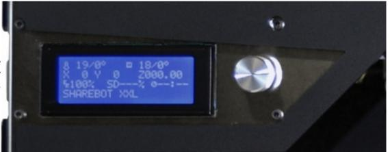
The third row has on the left the percentage control of speeds: turning the control knob we modify in percentage all the different speeds that are present in the gcode.
