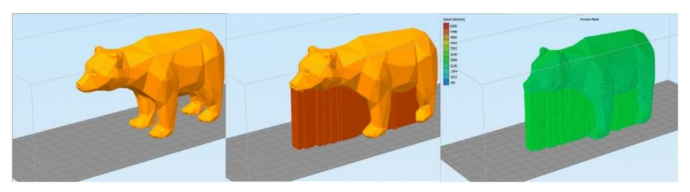
The support material are vertical structures generated -in this case – under the surfaces tilted over 45°.
