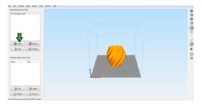
The second step is to click on the "Add" button in the left lower window. After pressing this button the "FFF window" pops up where you can select a standard print profile in the drop down menu.
