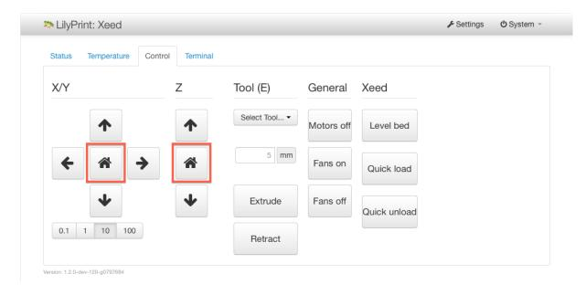
After this you can use the arrows to move the extruder head or the printer bed.
