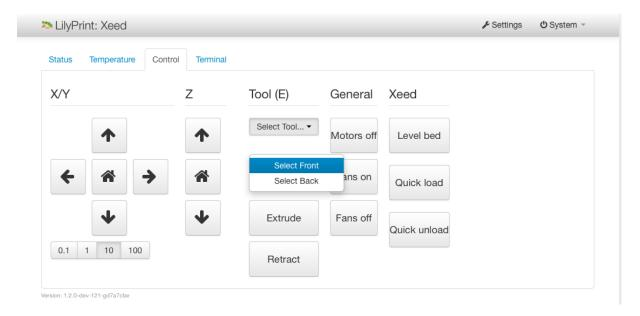
After pushing the Extrude button, the filament will be guided through the tube towards the extruder head and covers a small distance inside the tube each time you press this button. This is a good way clear your nozzles with newly molten filament before starting a new print.
