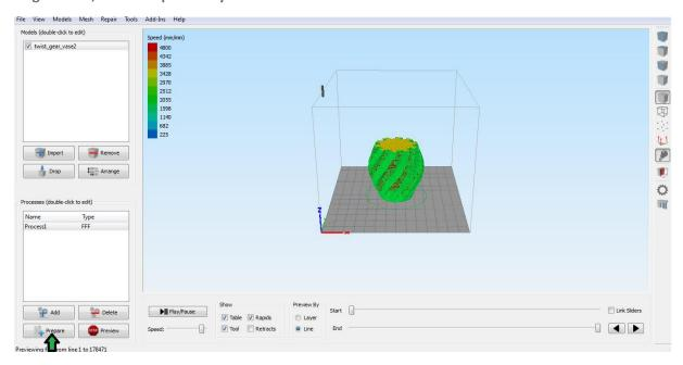
The G-code can now be uploaded by your printer through a computer connection as explained in paragraph "2.4.2. Uploading a model from your computer" and is ready to be printed!
