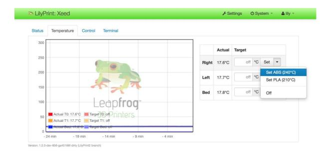
You can notice that the temperature graph of the front extruder shows the current and target temperature.
