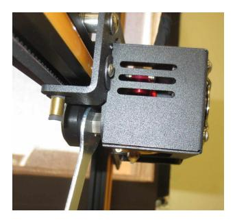
c. Re-check the tension of the nozzle assembly. The assembly and the belt should move left and right without much effort, but there should have no side-to-side wiggle or play.
