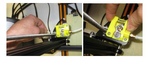
d. Push the filament all the way through the Bowden tube until it stops when it hits the back of the nozzle.
