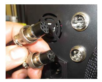
d. Connect the stepper motor and limit switch cables.
