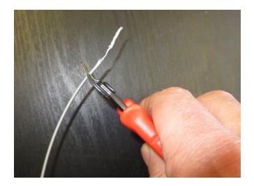
c. Feed the end of the filament into the extruder with one hand as you squeeze the extruder release lever with your other hand.
