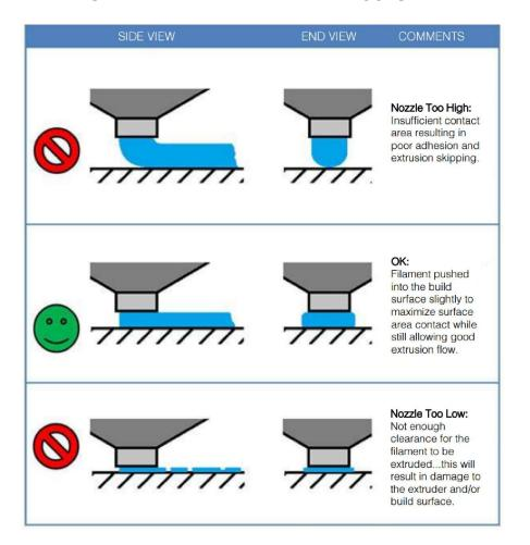
a. If the bed is too low, the extruded plastic may not stick to the build plate. Parallel lines of filament on the first layer will look rough, with high tracks and low valleys that are not stuck to the build plate.
