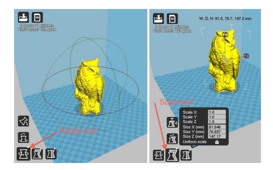
h. When you are satisfied with the Cura settings and the position, orientation, and scale of the model, select the "Save toolpath" (or "SD" if the microSD card is inserted) icon or File > Save GCode. Save the file to the microSD card that came with your printer.
