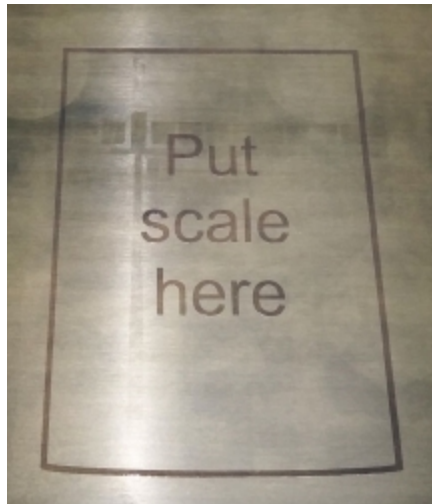
Figure 6-55 Scale positioning frame on the build tray
