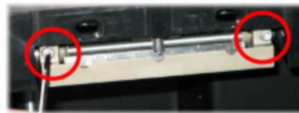
Figure 6-38 Removing the roller waste collector
