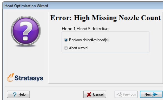
Figure 6-59 Head replacement due to missing nozzles
