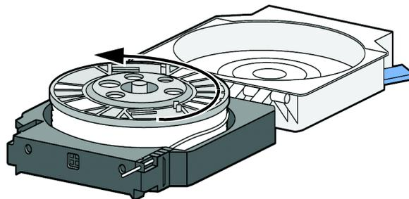
8. Using a cutters, cut the excess 2 inches (50mm) of material from the material guide. leaving a blunt end.
