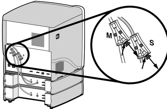
17. Connect the short red striped material tube (M1) from model (M) coupler of upper material bay to **left** side of model Y block by inserting firmly into red couplers. Gently pull the tube to ensure it is properly inserted.
