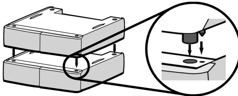
15. With 2 people, position the printer on to the top of the material bays. Be sure the feet and pins are properly aligned. See [Figure 3-4](#).
