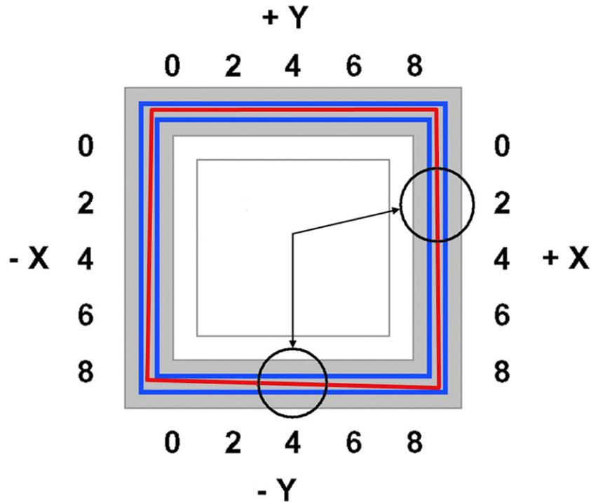
5. Select **Done** after you have input the X and Y offsets. The printer will return to **Maintenance**. Run the XY calibration a second time to be sure the values changed the offset properly.
