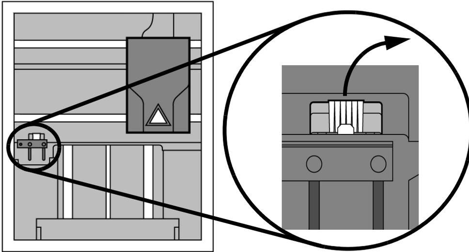
4. Place the new tip wipe assembly over the two mounting posts making sure the assembly is fully installed. See [Figure 5-4](#).
