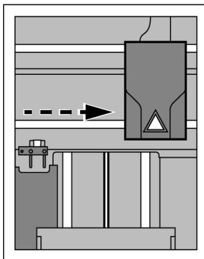
3. Remove the tip wipe assembly by lifting the assembly up and out of the printer. Discard this tip wipe assembly. See [Figure 5-3](#).
